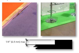
Changes in level greater than 1/4" (6.4 mm) high minimum and not more than 1/2" (13 mm) high maximum must be beveled with a slope not steeper than 1:2. A change in level of 1/2" (13 mm) is permitted to be 1/4" (6.4 mm) vertical plus 1/4" (6.4 mm) beveled. But, the combined change in level may not exceed 1/2" (13 mm). To prevent tripping, beveled slopes must be made of solid material.
