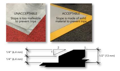
Changes in level greater than 1/2" (13 mm) are required to be ramped. To accommodate the widest range of users, ramps should have the least possible running slope, which may not be steeper than 1:12.
